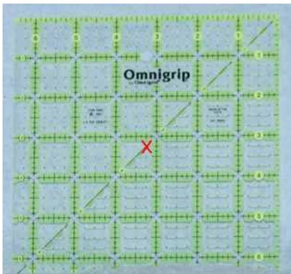
This Omnigrip ruler has the 1/2 on the left side and at the bottom. The red x indicates where the center is on this ruler. Notice that it is NOT at the cross mark of the ruler lines..
